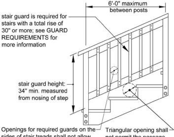
sides of stair treads shall not allow a sphere 4-3/8" to pass through.
