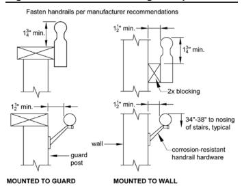
than 6- $\frac{1}{4}$ ". Type II rails with a perimeter greater than 6- $\frac{1}{4}$ " shall provide a graspable finger recess area on both sides of the profile [R311.7.7.3]. All shapes shall have a smooth surface with no sharp corners. Handrails shall run continuously from a point directly over the lowest riser to a point directly over the highest riser and shall return to the guard at each end (see Figure 33). Handrails may be interrupted by guard posts at a turn in the stair [R311.7.7.2].
